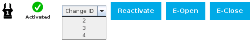
Fig. 4-10: Gripper ID modification in the Gripper Dashboard
