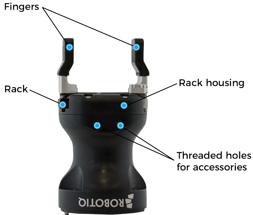
Fig. 1-1: Robotiq Hand-E Gripper.
