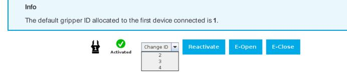
Fig. 4-11: Gripper ID modification in the Gripper Dashboard
