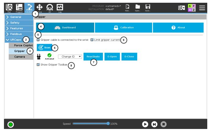
Fig. 4-8: Gripper Dashboard (steps highlighted)
