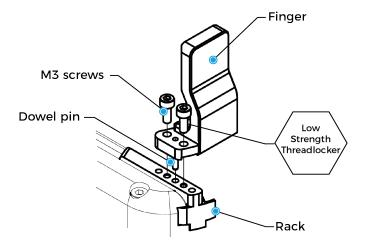
Fig. 3-7: Mounting fingers on racks.
