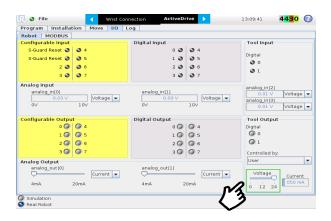
Fig. 8-3: Voltage set to 24V.
