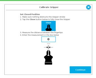
Fig. 4-17: First step of the calibration wizard
