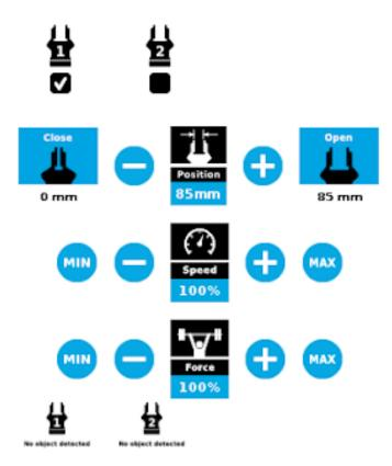
Fig. 4-25: Gripper Toolbar (expanded, multiple grippers)
