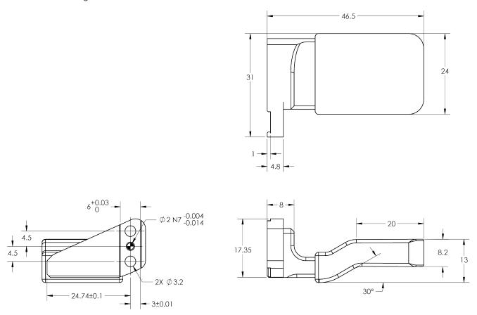
Fig. 5-6: Flat NBR overmolded finger.
