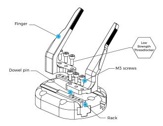
Fig. 3-10: Mounting bin picking fingers on racks.
