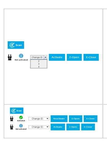
1. Check that gripper ID is different from that of other grippers that will be connected to the robot, and if required, select a different ID from the "Change ID" dropdown list.
