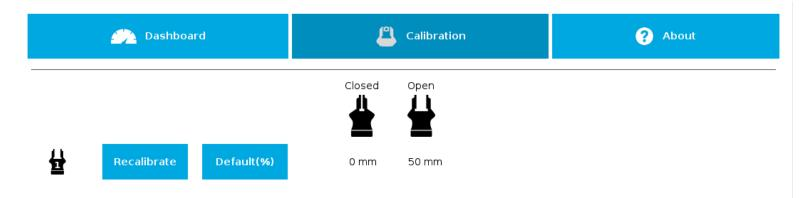
Fig. 4-19: Single Gripper, calibrated
