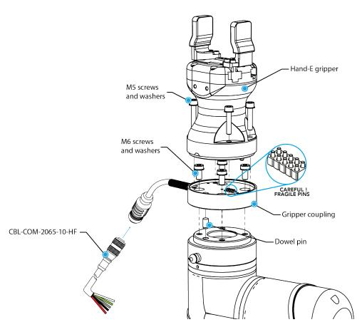
Fig. 3-1: Installing Hand-E on the robot tool flange for CB-Series.
