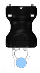
Fig. 5-12: Friction grasp and form-fit grasp.
