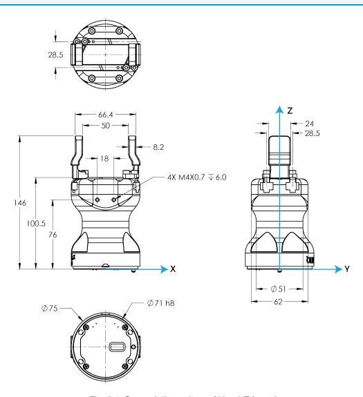
Fig. 5-1: General dimensions of Hand-E (open).
