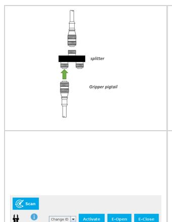
1. Connect only one gripper at a time using the splitter.
