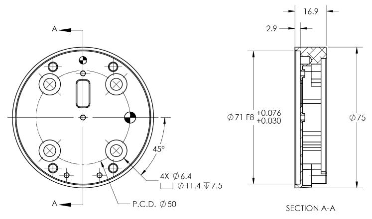
Fig. 5-2: Coupling for ISO 9409-1-50-4-M6.
