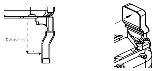
Fig. 5-10: Z-axis offset at which force/payload is applied.
