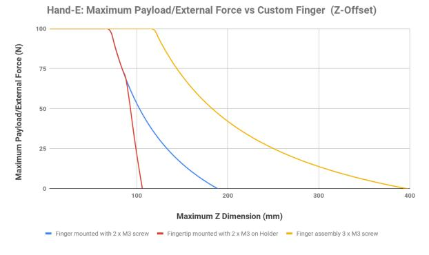
Fig. 5-11: Graph illustrating Maximum Payload/External Force vs. Z-Offset on Custom finger.
