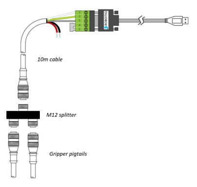
Fig. 3-13: Multiple grippers wiring.
