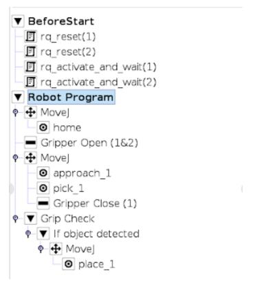
Fig. 4-30: Example of UR script commands with multiple Grippers
