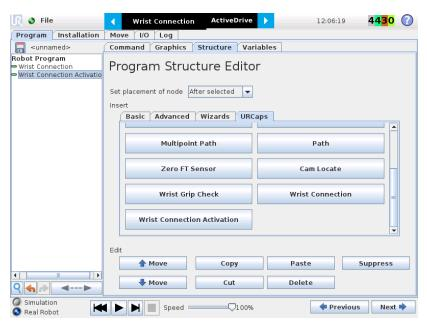
Fig. 4-3: Program Structure Editor. Multiple Wrist nodes are available.
