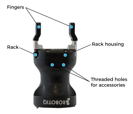
Fig. 1-1: Robotiq Hand-E Gripper.
