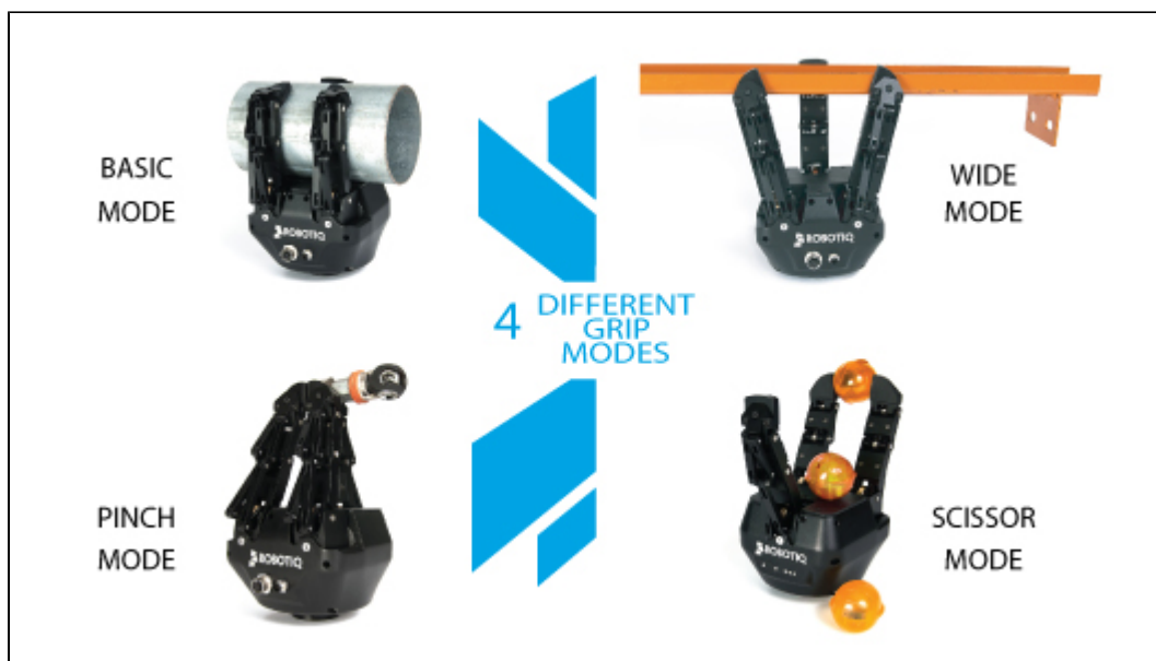
Figure 1.3 – The four Operation Modes of the Adaptive Gripper.
