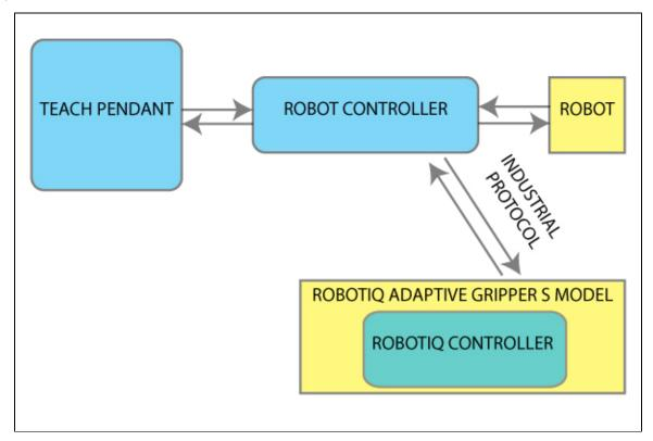
Figure 4.1.1: Adaptive Gripper S-Model connections.
