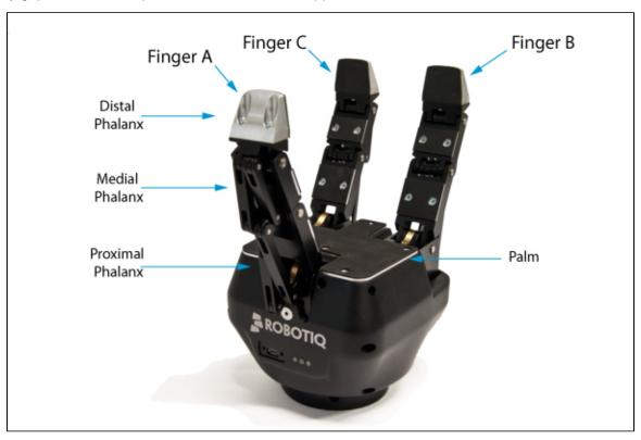
Figure 1.1: The Adaptive Gripper S model.
