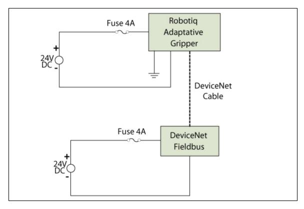
Figure 3.4.2.2 : Power connection diagram of the Adaptive Gripper S-Model using DeviceNet Fieldbus.
