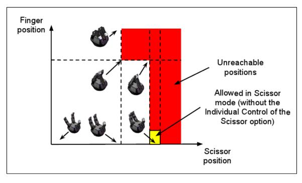
Figure 4.6.1: Reachable workspace of the fingers and scissor axis.
