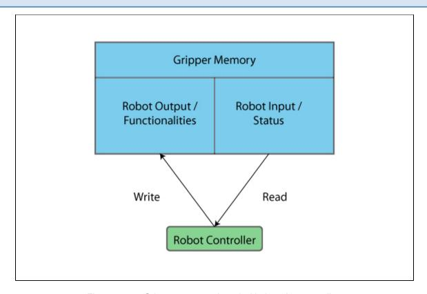
Figure 4.3.1 : Gripper memory shared with the robot controller.
