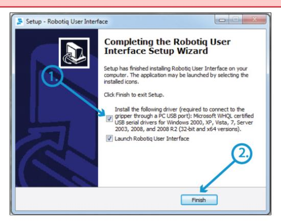
Figure 5.2.1: Completing the installation of Robotiq User Interface
