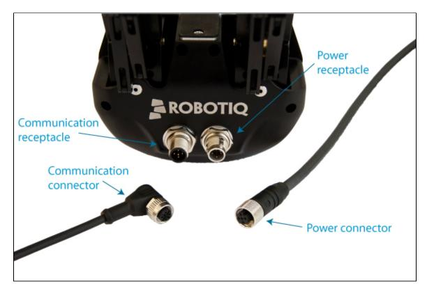
Figure 3.4.1: Power and Communication receptacles and connectors.
