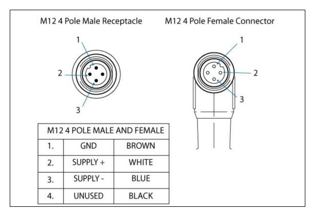
Figure 3.4.1.2 : Gripper Power Inlet and Power Connector.
