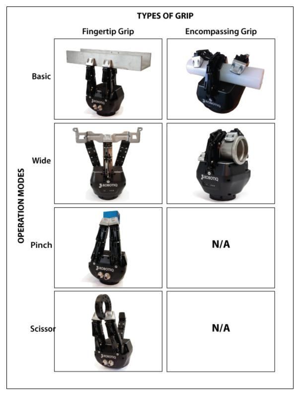
Figure 1.6 : Operation Modes vs. Types of Grip.
