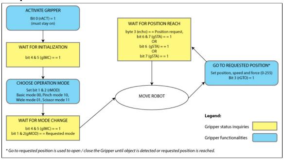
Figure 4.8.1: Example of Adaptive Gripper S model registers.
