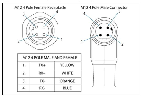
Figure 3.4.2.4: Real-time Ethernet communication pin-out.
