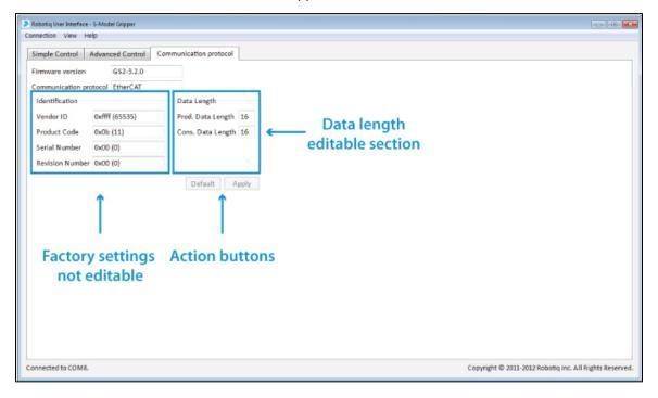
Figure 5.6.5.1: Default screen of the Configuration Tool with EtherCAT
