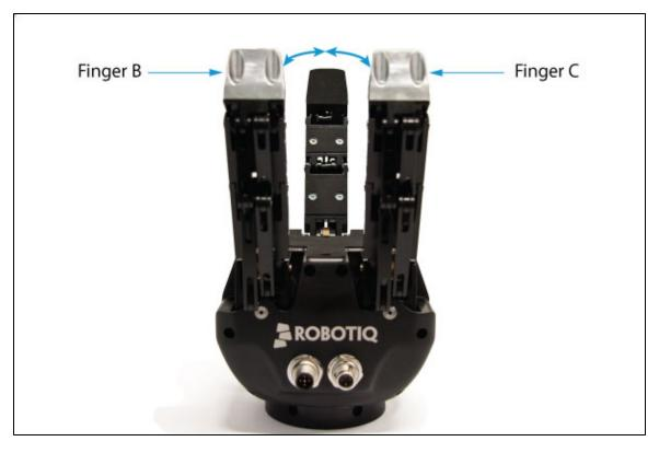
Figure 1.2: First type of movement of the Adaptive Gripper S model: changing the Operation Mode
