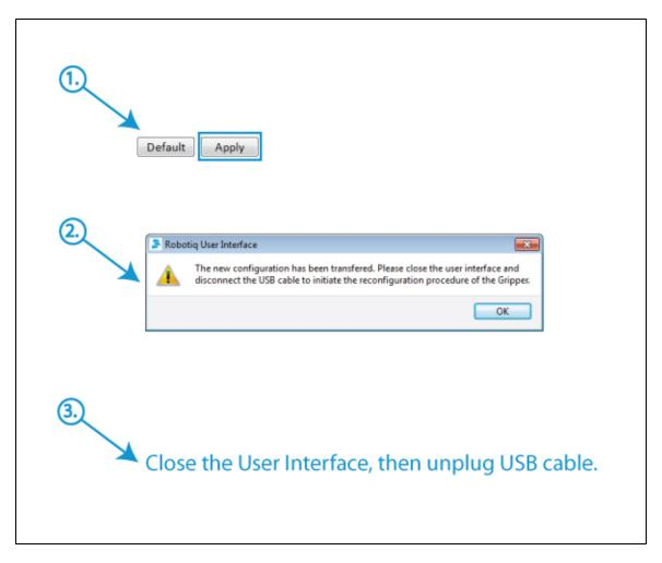
Figure 5.6.2 : Applying changes to the communication protocol settings.
