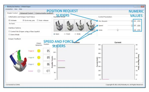
Figure 5.4.4.1: Changing the Control Parameters of the Gripper
