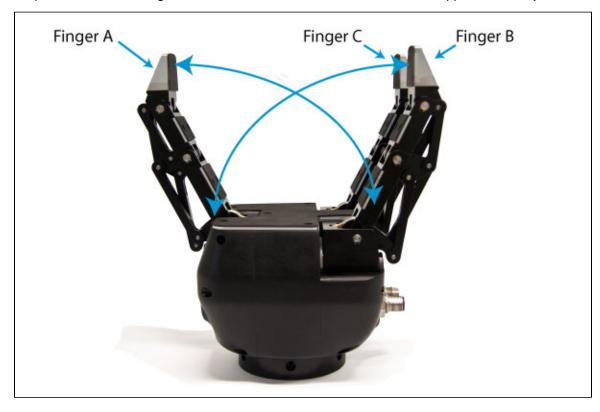
Figure 1.4: Second movement of the Adaptive Gripper S model: closing and opening the fingers.
