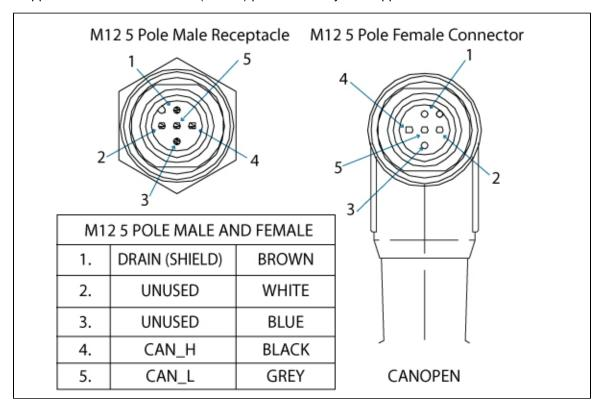
Figure 3.4.2.3: CANopen communication pinout.
