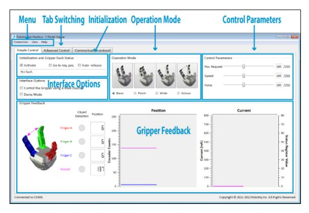
Figure 5.3.2 Gripper Simple Control tab description.
