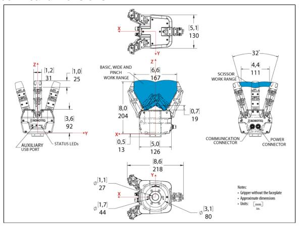
Figure 6.1.1: Robotiq Adaptive Gripper model S technical dimensions.
