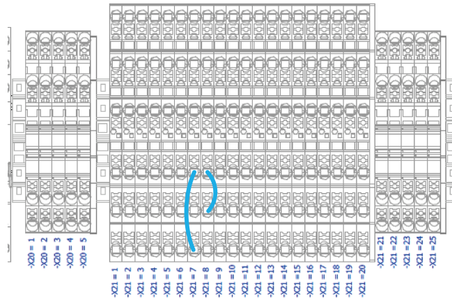
Fig. 6-6: Example of Jumpers Connections
