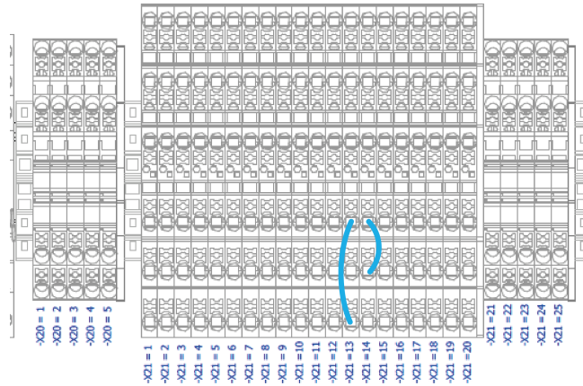
Fig. 6-9: Example of Jumpers Connections
