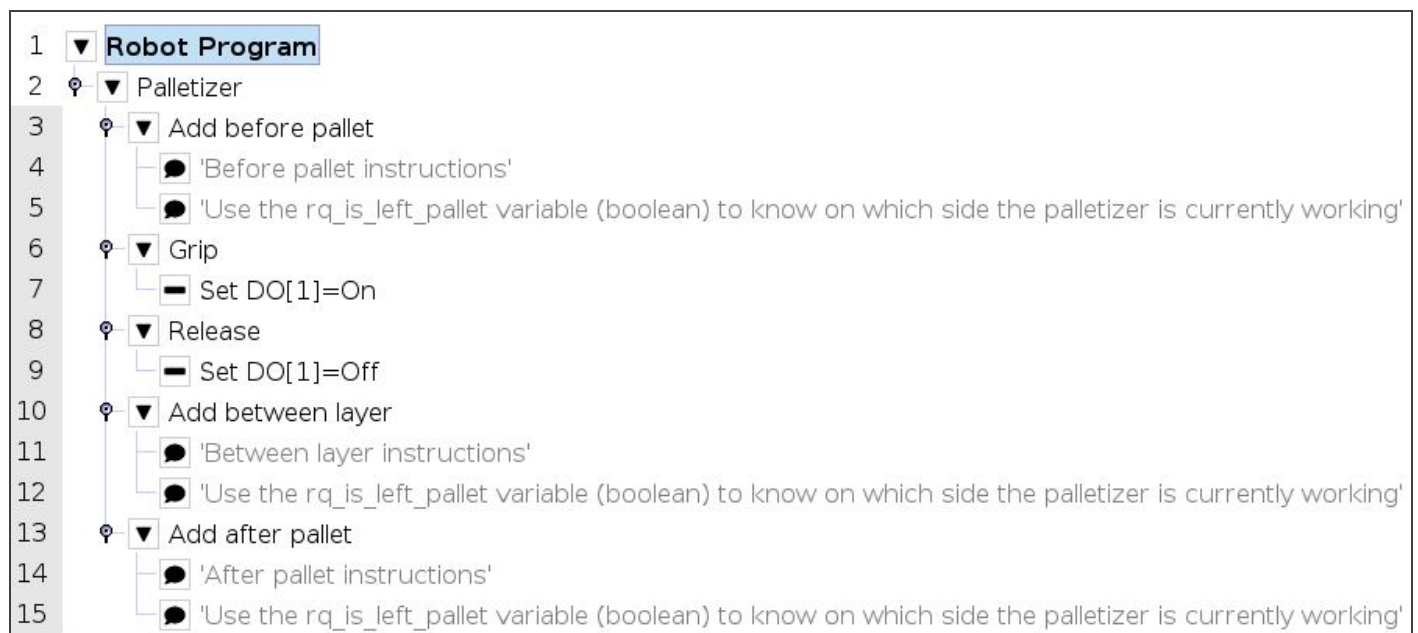
Fig. 5-26: Standard Palletizer Node in a Program Tree
