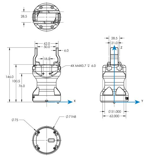
Fig. 8-1: General dimensions of Hand-E (open).
