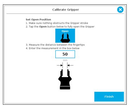
Fig. 4-5: Second step of the calibration wizard
