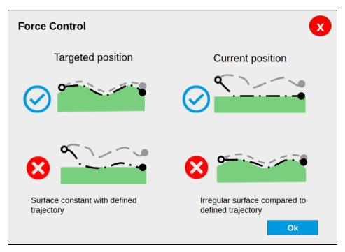
Fig. 5-21: Tooltip illustrating when to use a type of position, and when to avoid using it.
