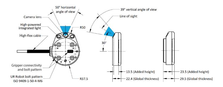
Fig. 8-5: Hardware of the Wrist Camera.
