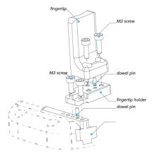
Fig. 1-3: Mounting a fingertip on a fingertip holder (example).
