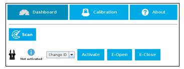
Fig. 3-5: Activating a gripper and assigning and ID.
