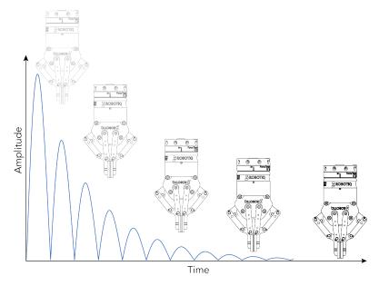
Fig. 5-19: An end-effector meets adaptive stiffness upon repeated contacts with a surface.
