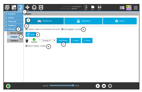
Fig. 4-1: Gripper Dashboard (steps highlighted)
