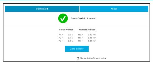
Fig. 5-16: The Force Copilot dashboard displays force and torque values in real time.
