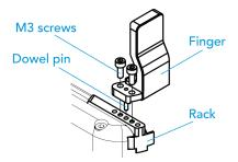
Fig. 1-2: Mounting a finger on a rack.
