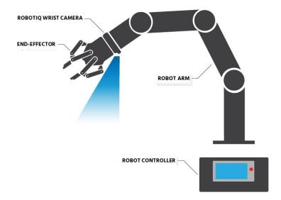
Fig. 1-8: Schematic representation of the Robotiq Wrist Camera Vision System hardware.
