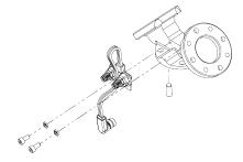
Fig. 3-2: Securing the M8 splitter to the adapter plate.
