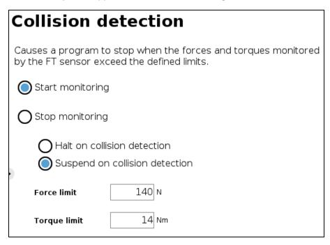
The Collision Detection feature in the Installation tab can be configured to start the monitoring upon every robot program start. On the other hand, the Collision Detection node in the Program tab starts a thread that runs in parallel with the rest of the robot program. If the Stop monitoring option is selected in the Collision Detection node, the thread stops and the program continues without monitoring the force or the torque.
