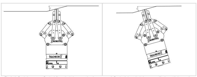
Fig. 5-18: Deviation range - On the left, no deviation range has been entered. On the right, a deviation range of at least 15 degrees has been entered around the corresponding axis.
