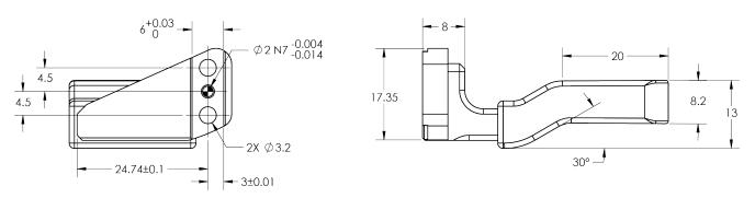
Fig. 8-4: Flat NBR overmolded finger is mounted on Hand-E by default.
