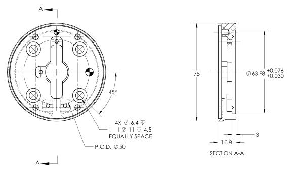
Fig. 8-2: Coupling for ISO 9409-1-50-4-M6.
