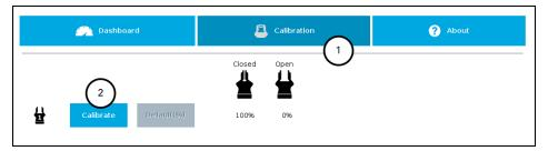
Fig. 4-3: Calibrating grippers.
