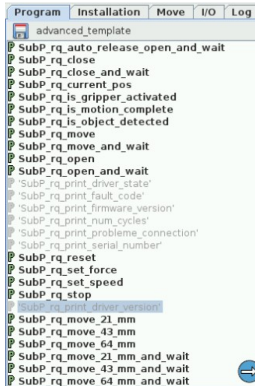
Fig. 4-25: Older program's subprograms to suppress or rename to use with URcaps package.
