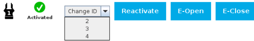
Fig. 4-4: Gripper ID modification in the Gripper Dashboard
