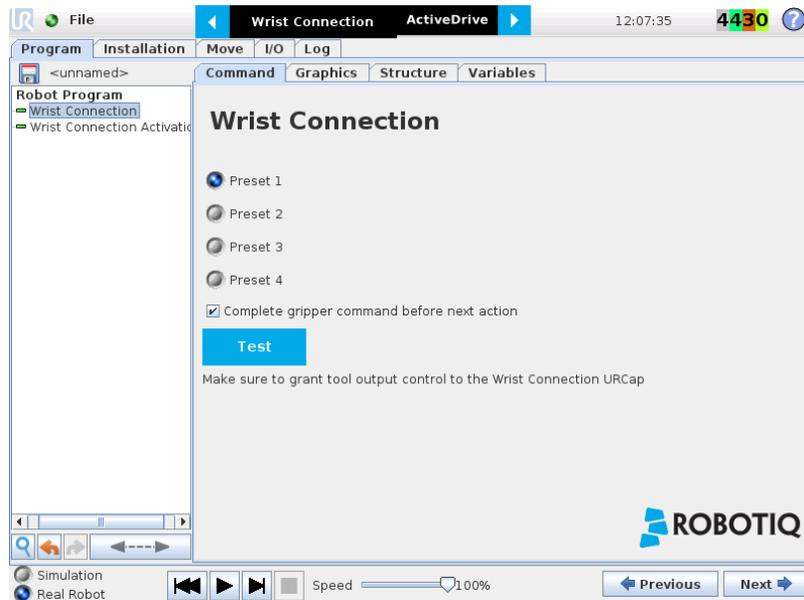
Fig. 4-5: Wrist Connection Node Interface.
