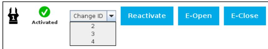
Fig. 4-9: Gripper ID modification in the Gripper Dashboard
