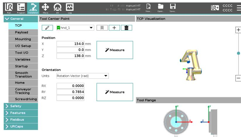
Fig. 4-8: TCP Menu in the PolyScope Interface
