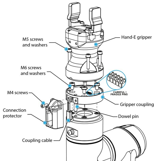
Fig. 3-18: Installing the Hand-E on the robot tool flange
