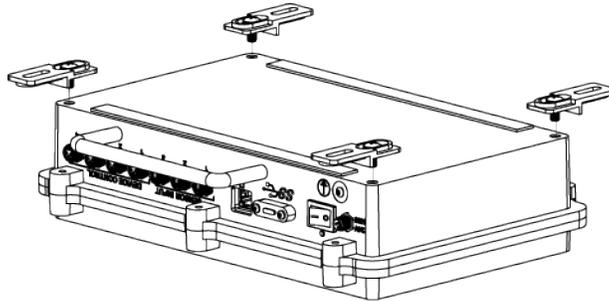
*Fig. 3-6: Installing the brackets under the Robotiq controller*
