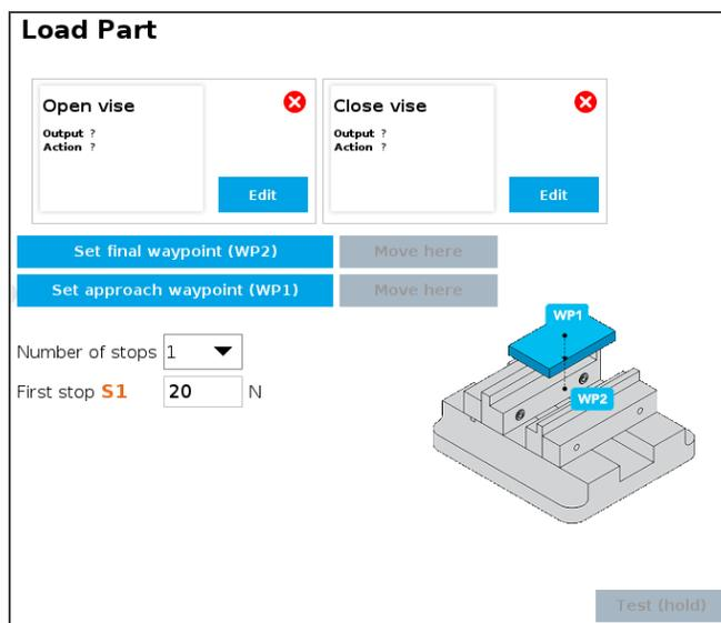
1. Tap **Open vise**. Select the according **Digital output** and the **Action** to open the vise. Tap the home icon to go back to the Load Part node. This might be already configured if you named the Digital output work\_open in **Robotiq Controller Configuration** section
