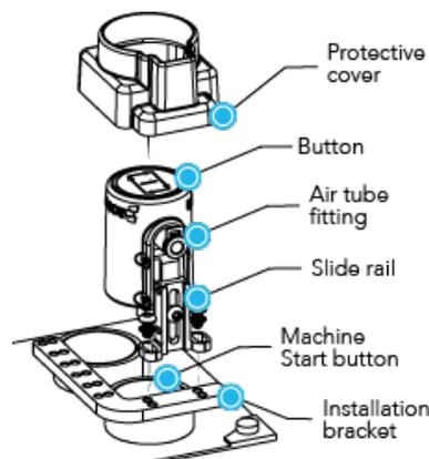
Fig. 3-13: Installing the Button Activator
