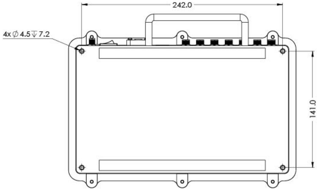
Fig. 5-13: Robotiq Controller technical dimensions - bottom view
