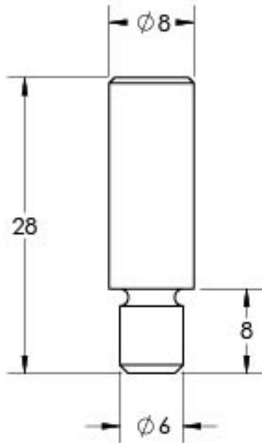
*Fig. 5-6: Large Pin technical dimensions*
