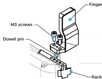
Fig. 3-23: Installing the Flat Overmolded Fingertips on the racks
