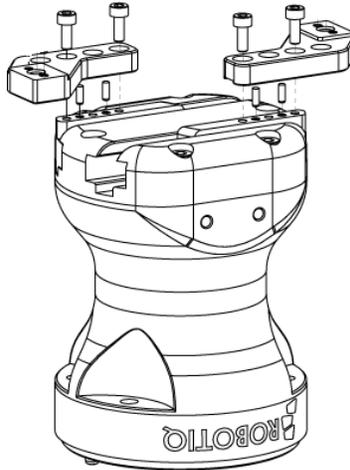
*Fig. 3-24: Installing the Adjustable Fingertip Holders*
