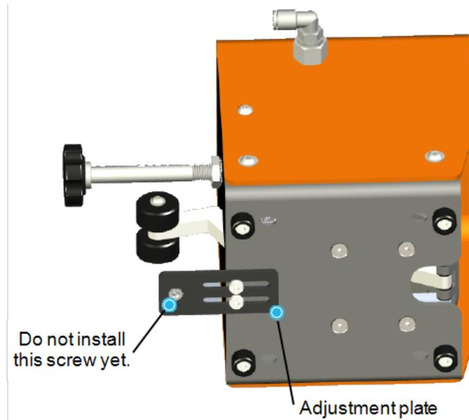
*Fig. 3-43: Installing the adjustment plate*
