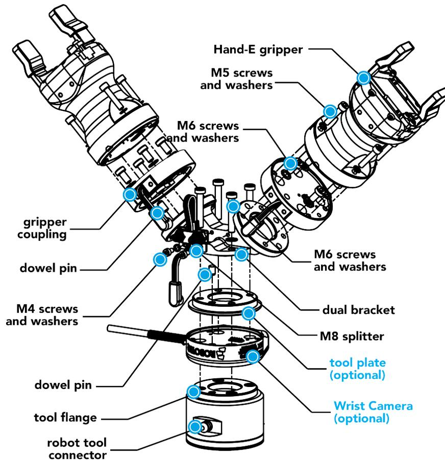
Fig. 3-19: Installing Dual Hand-E Gripper on Dual Bracket
