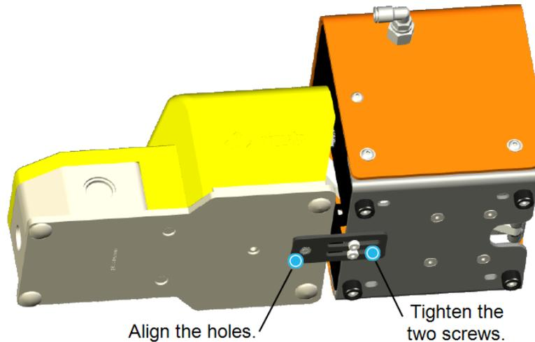
Fig. 3-45: Adjusting the position of the adjustment plate
