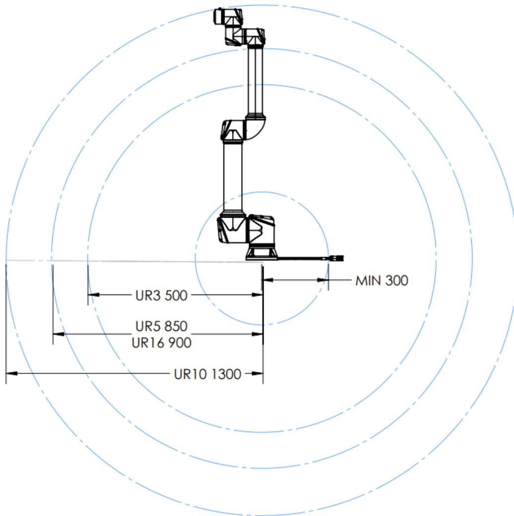
Fig. 3-2: Minimum and maximum distances from robot's center
