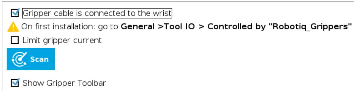
Fig. 4-2: *Gripper cable is connected to the wrist* check Box.
