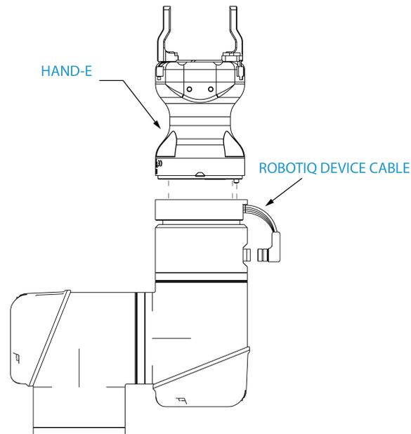
Fig. 3-50: Robotiq Hand-E with device cable wiring scheme
