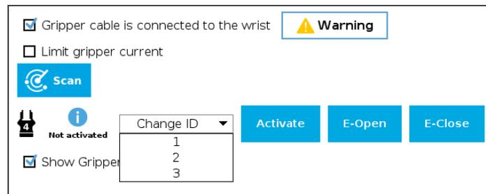
Fig. 4-6: Verifying each Gripper has a different ID
