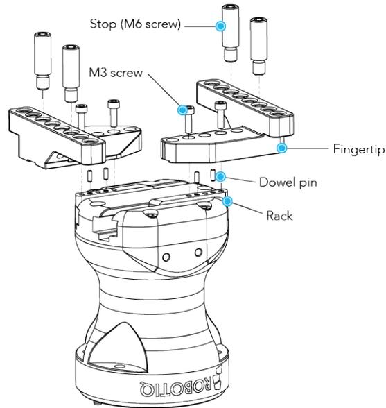
Fig. 3-29: Installing the 4 Stop Fingertips
