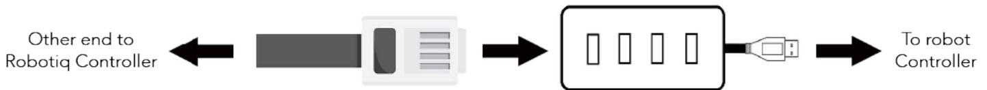
Fig. 3-48: Connecting Robotiq Controller's Ethernet cable to the robot controller
