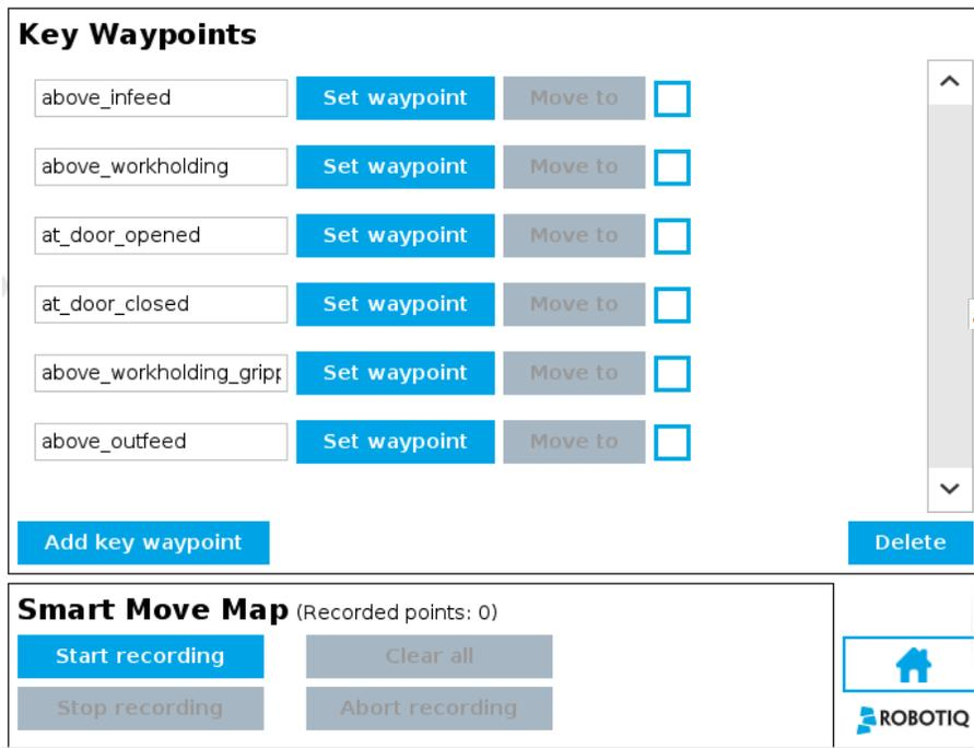
Fig. 4-19: Recording the **Smart Move Map**
