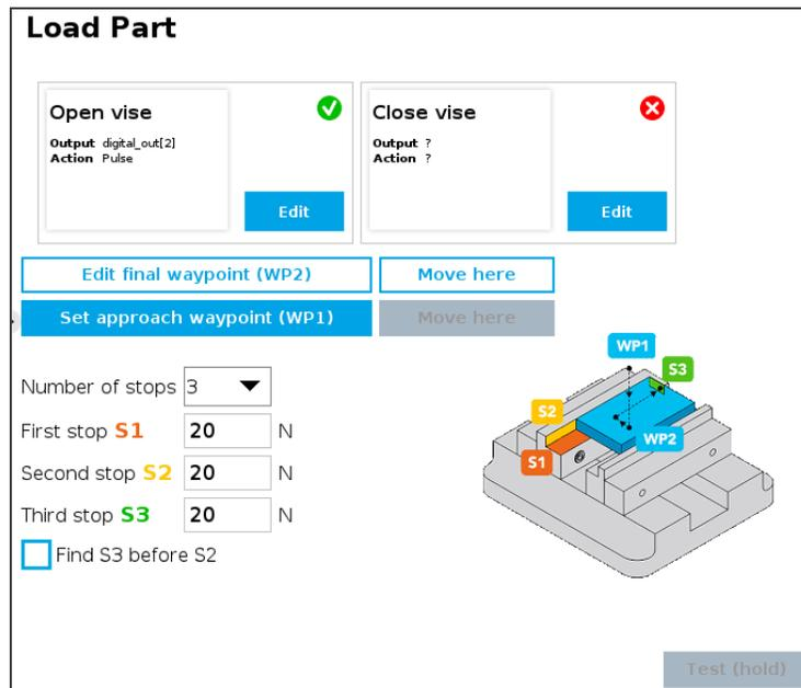
5. Set the approach waypoint as follow. Use the **TCP Position** feature as per **Software** section to move the robot, as the alignment with the final waypoint must not be lost.
