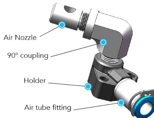
*Fig. 3-32: Air Nozzle assembly*
