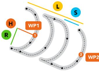
The diagram illustrates a curved pattern of three parallel, semi-circular paths. Two waypoints, WP1 and WP2, are marked at the start and end of the pattern. Parameters are labeled: H (Height) is the vertical distance between the top of the curves; R (Radius) is the radius of each curve; L (Length) is the distance between WP1 and WP2; and S (Spacing) is the distance between adjacent curves. Arrows indicate the direction of movement along the curves.
