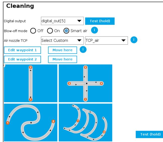
4. Set **waypoint 1** and **waypoint 2**. Those two waypoints will be set for any cleaning pattern you will select. The air nozzle must be perpendicular to the workholding and at the same distance from it when setting the waypoints.
