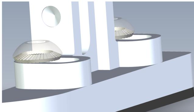
*Fig. 3-14: Orientation of the M3 washers*
