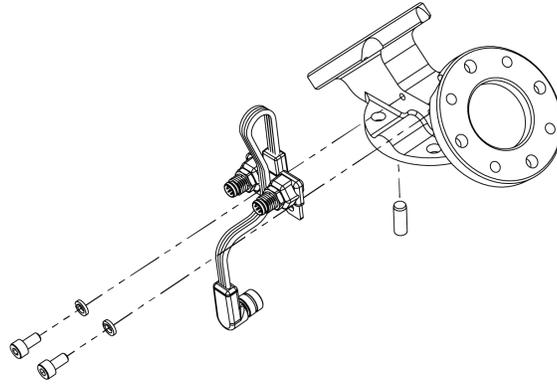
Fig. 3-22: Fastening the M8 splitter to the Bracket
