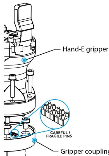
Fig. 3-21: Carefully align the small fragile pins
