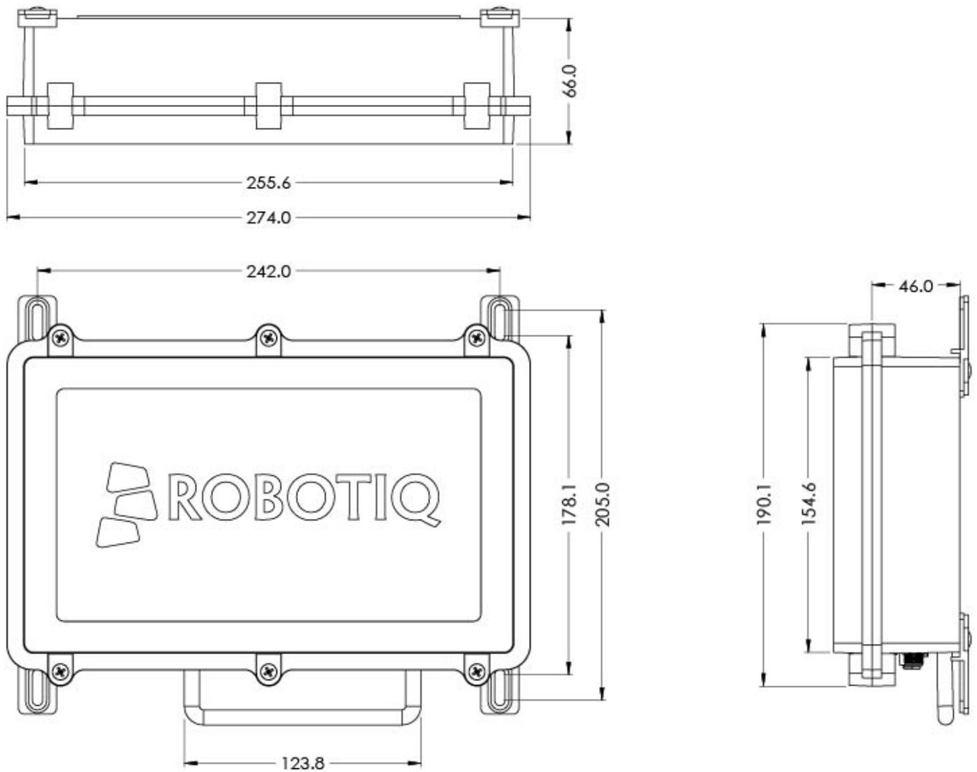
Fig. 5-12: Robotiq Controller technical dimensions
