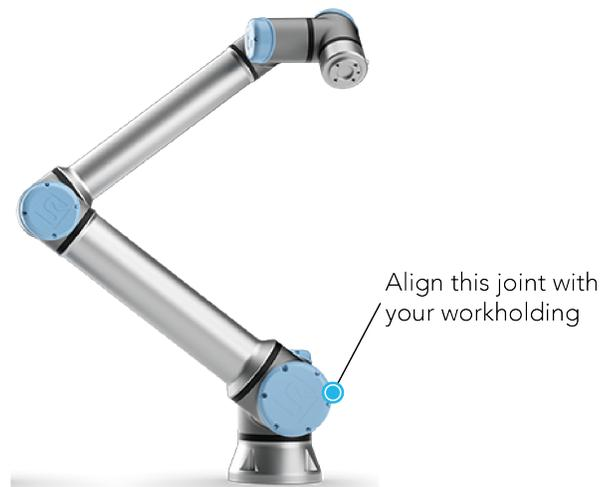
*Fig. 3-4: Set the height of the robot*
