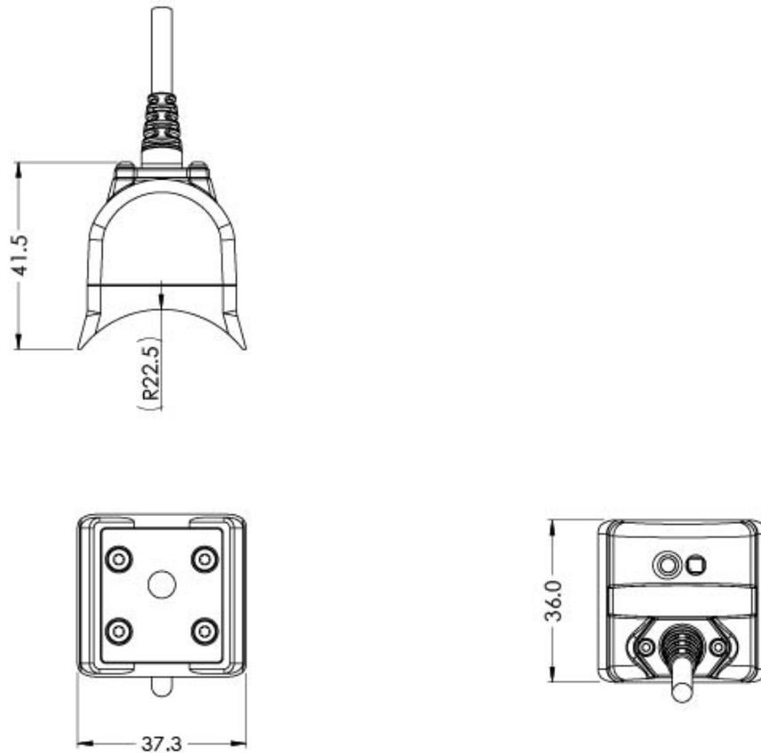
Fig. 5-14: Stacklight Monitoring Sensors technical dimensions
