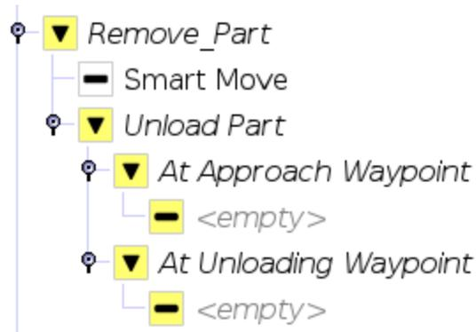
Fig. 4-31: unload\_part node in program tree
