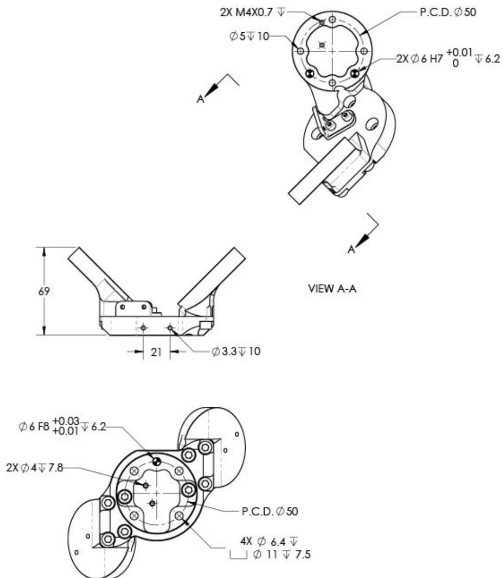
Fig. 5-16: Compact Dual Hand-E Bracket technical dimensions
