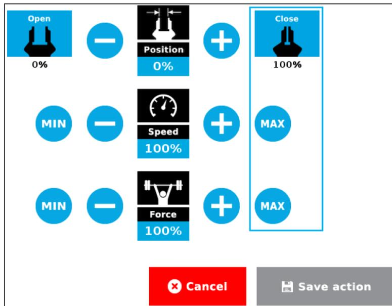
Fig. 4-16: Closing the gripper
