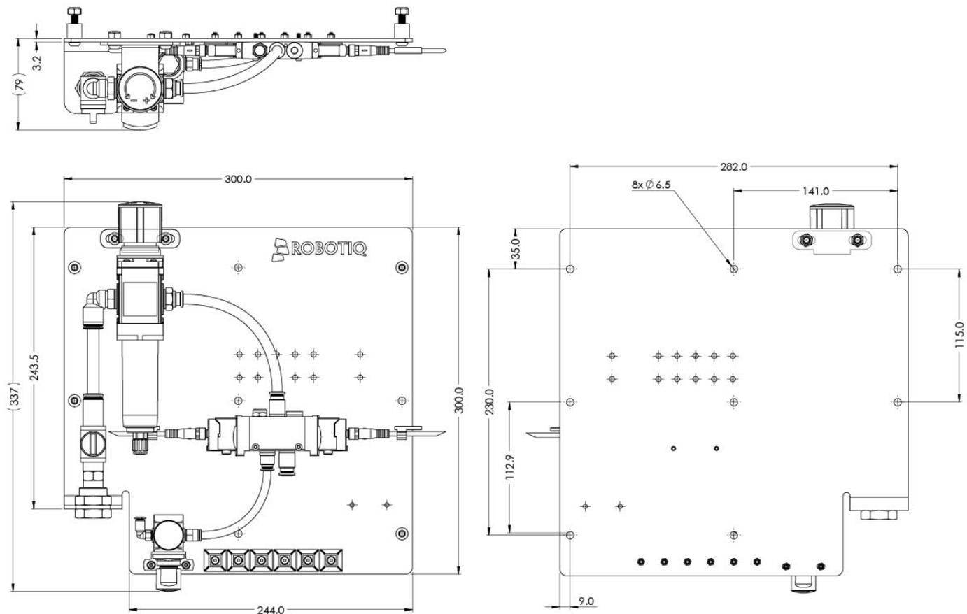
Fig. 5-11: Pneumatic Panel technical dimensions
