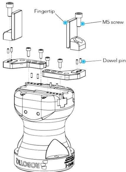
*Fig. 3-27: Installing the Flat Overmolded Fingertips on the Adjustable Holders*
