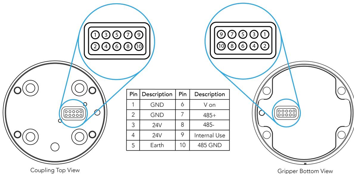
Fig. 3-49: Pinout to the Hand-E Gripper cable-to-wrist coupling.
