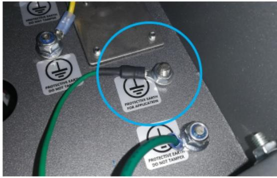
*Fig. 3-7: Connecting the protective earth cable in the robot controller*
