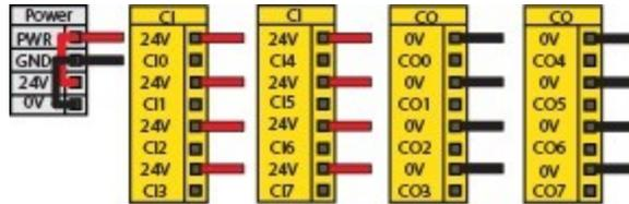
Fig. 3-52: Connecting the Wrist Camera to the robot controller
