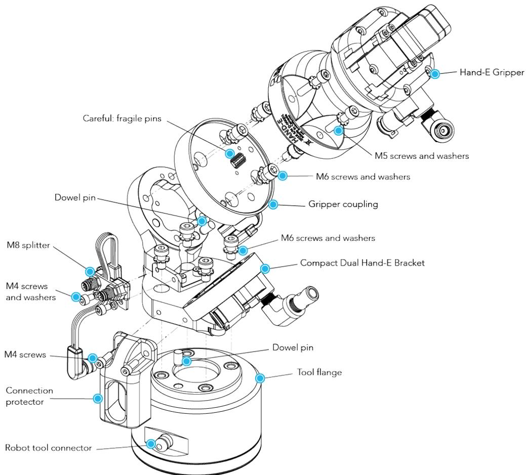
Fig. 3-20: Installing Dual Hand-EGripper on Compact Dual Hand-EBracket (only one Gripper shown)
