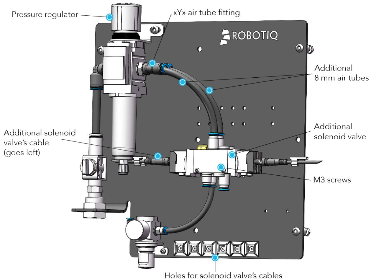
*Fig. 3-42: Assembling the pneumatic components for the Foot Switch Activator 1*
