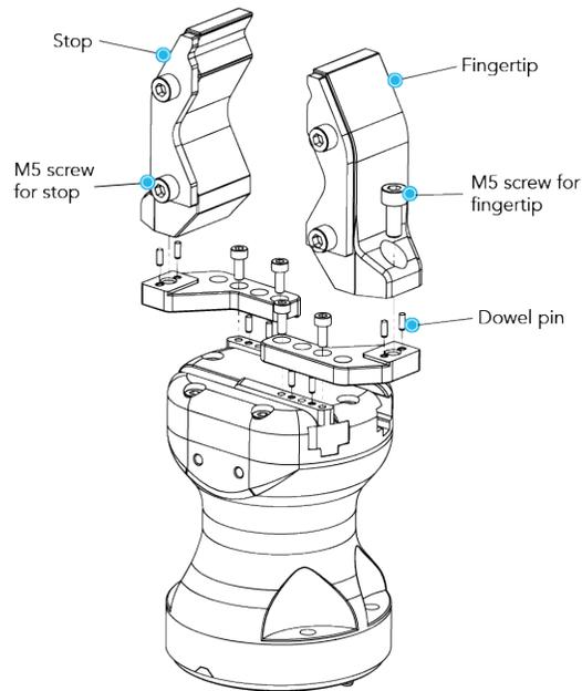
Fig. 3-28: Installing the Small Radial Fingertips
