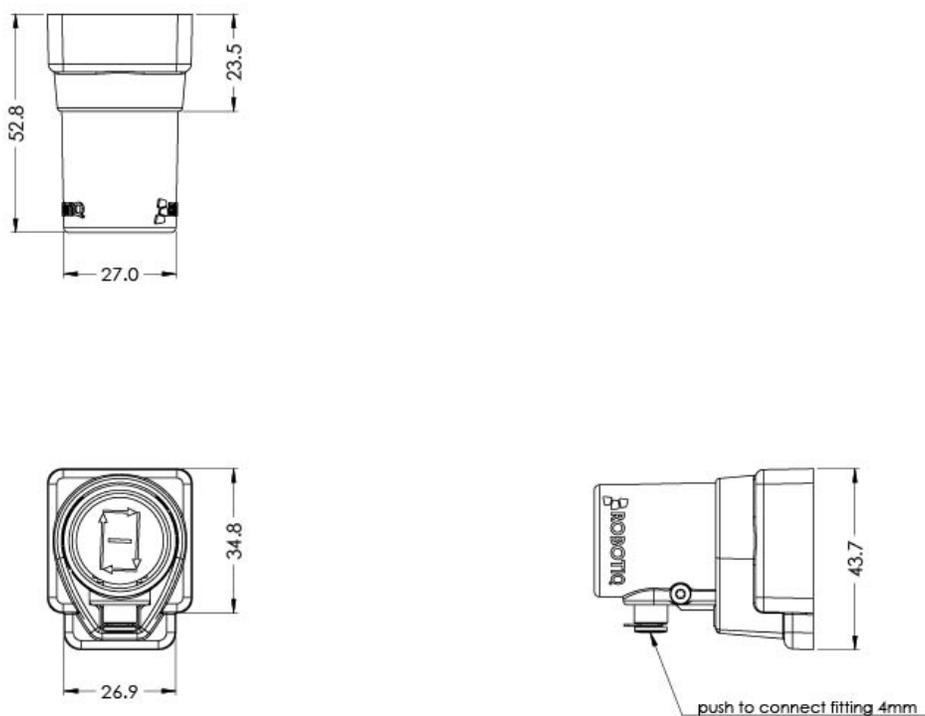
Fig. 5-1: Button Activator technical dimensions
