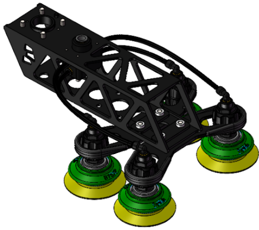
Fig. 3-14: 200 mm tube with small and large suction cup brackets
