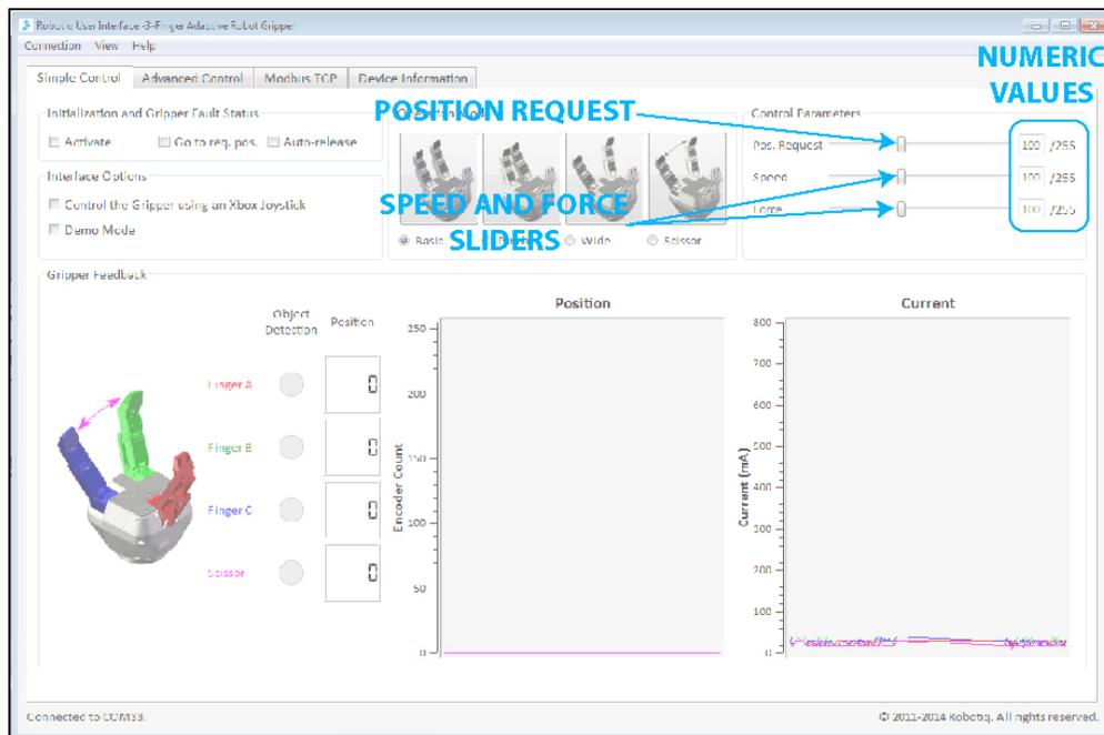
Figure 5.1.4.1 : Changing the Control Parameters of the Gripper
