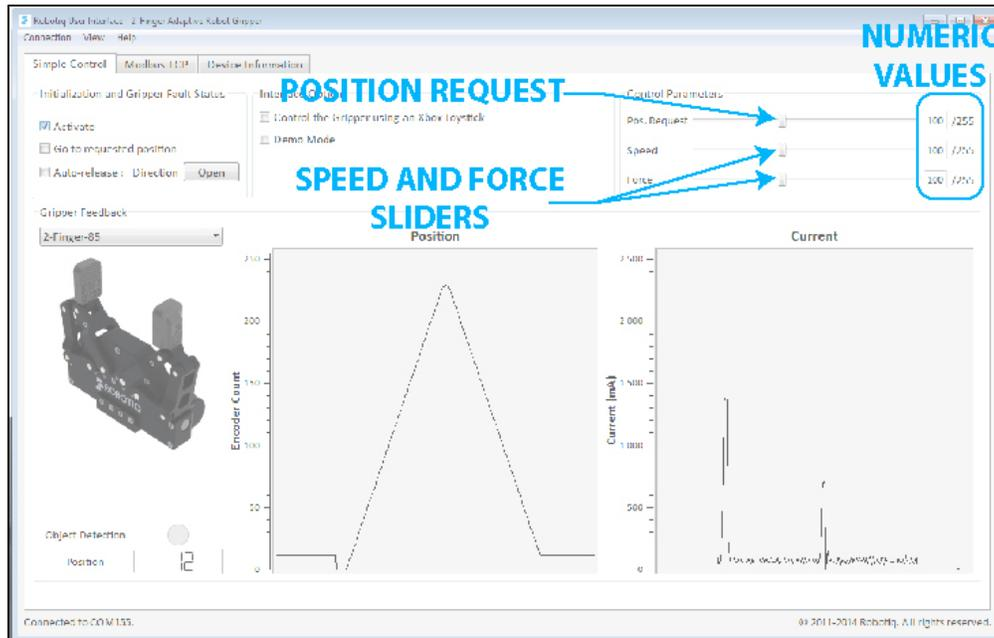
Figure 5.2.3.1 : Changing the Control Parameters of the Gripper
