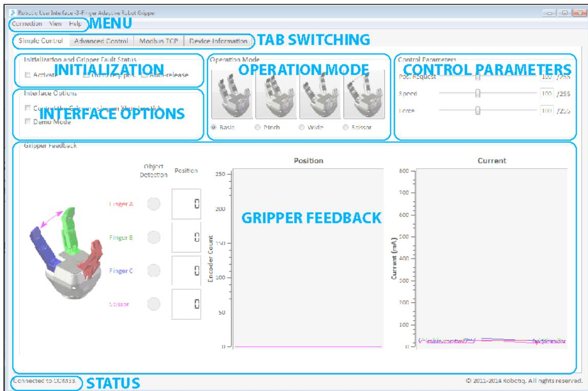
Figure 5.1.1 Gripper Simple Control tab description.
