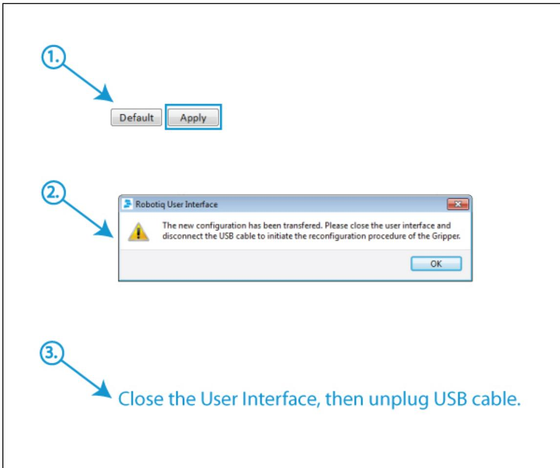
Figure 6.2 : Applying changes to the communication protocol settings.
