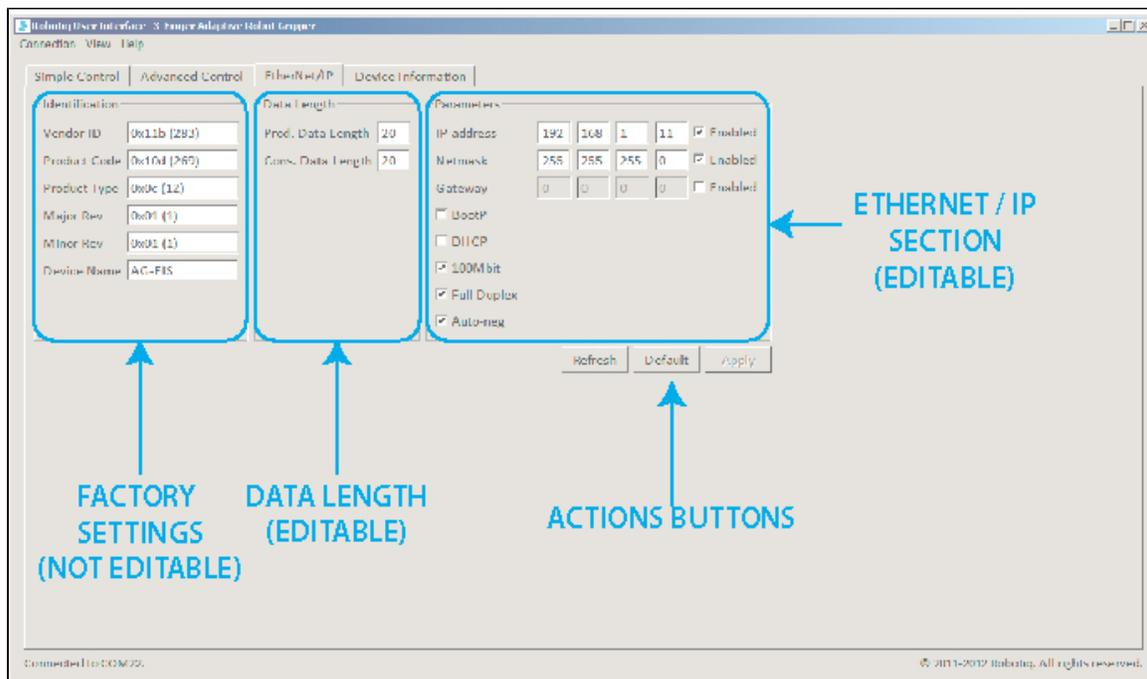
Figure 6.1.1 : Default screen of the Configuration Tool with Ethernet/IP
