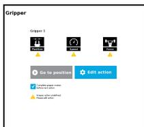
When the node is not defined, the Command window shows warning messages. Tap **Edit action** to modify the Gripper's action.
