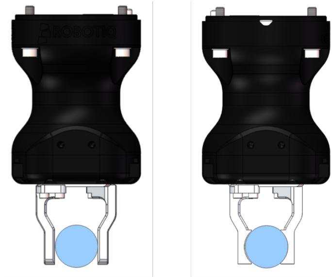
Fig. 8-9: Left: friction grasp; right: form-fit grasp.
