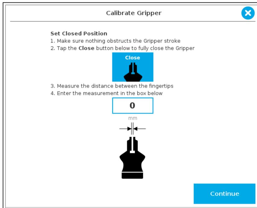
Fig. 4-4: First step of the calibration wizard
