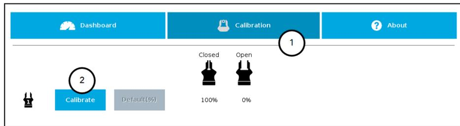
Fig. 4-3: Calibrating grippers.
