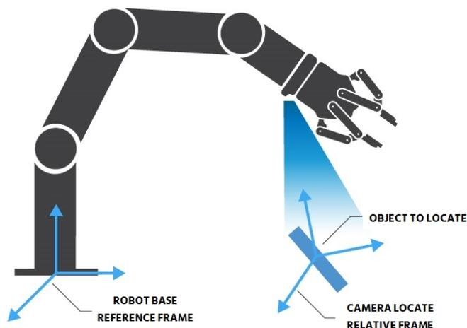
Fig. 1-10: Diagram of the object location process.
