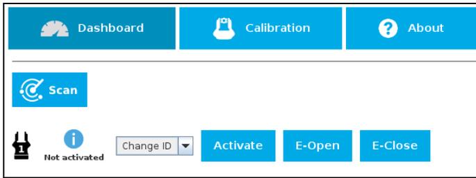
Fig. 3-5: Activating a gripper and assigning an ID.
