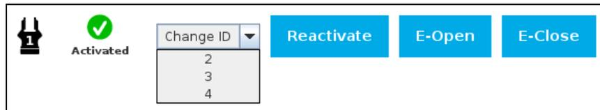
Fig. 4-2: Gripper ID modification in the Gripper Dashboard
