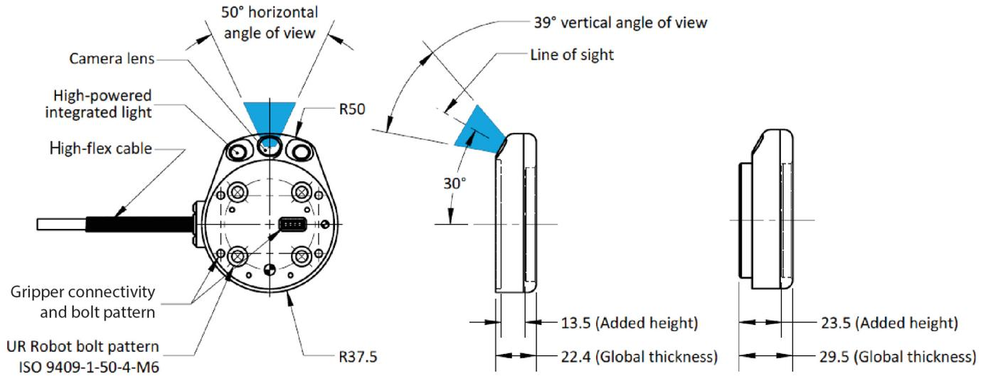
Fig. 8-5: Hardware of the Wrist Camera.
