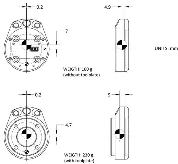
Fig. 8-6: Dimensions and weight of the Wrist Camera.
