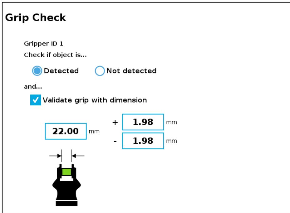
Fig. 4-12: Grip Check node interface with dimension validation
