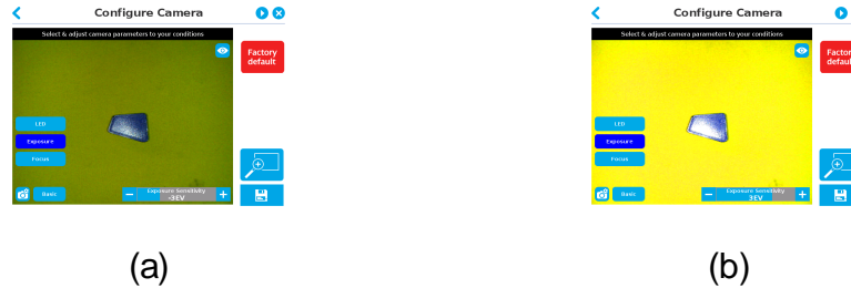
Fig. 7-10: Select Model step with Exposure option enabled (Basic mode); (a) -3EV and (b) 3EV
