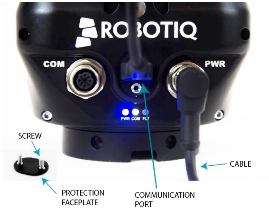
Figure 3.2.1 : Completed USB connection of the 3-Finger Adaptive Robot Gripper.
