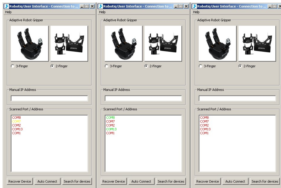
Figure 4.2 Scanning for device (left), device found (middle) and no device found (right).
