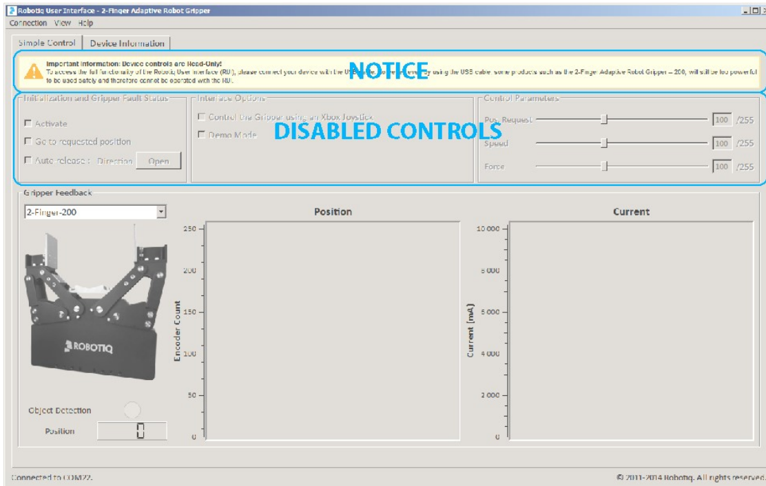
Figure 5.2.1 : The Simple Control tab is disabled for the Robotiq User Interface of the 2-Finger-200 or any Gripper when connected via Modbus TCP.
