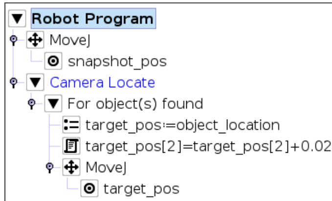
Fig. 4-72: Program example – Place the TCP 20 cm above the detected object, in case of an horizontal plane. e-Series robot program is illustrated.
