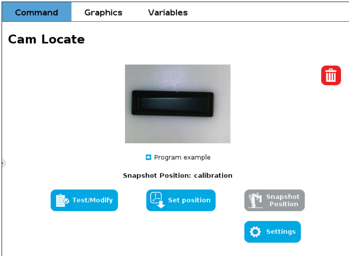
Fig. 4-73: The taught object model can be viewed from the "Command" tab of a Cam Locate node.
